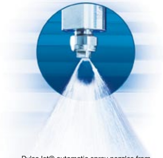
Pulsajet® automatic spray nozzles from Spraying Systems Co. are suitable for PWM flow control. Pulsajet nozzles operate at flow rates up to 59.8 L/min (15.8 gpm) and fluid pressures up to 24 bar (350 psi). Available with hydraulic or atomizing spray tips in a variety of spray patterns, Pulsajet nozzles can achieve cycle speeds up to 10,000 cycles per minute.
